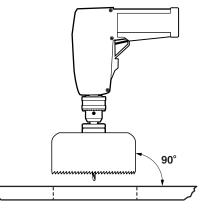
Figure 2-3 — Cutting the opening with a hole saw
